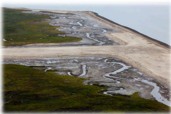
Figure 26: Aerial View of completed excavation to create wetlands
