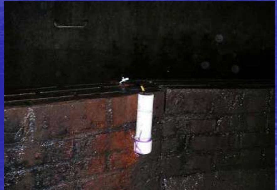
Pressure Sensor installed on weir wall
