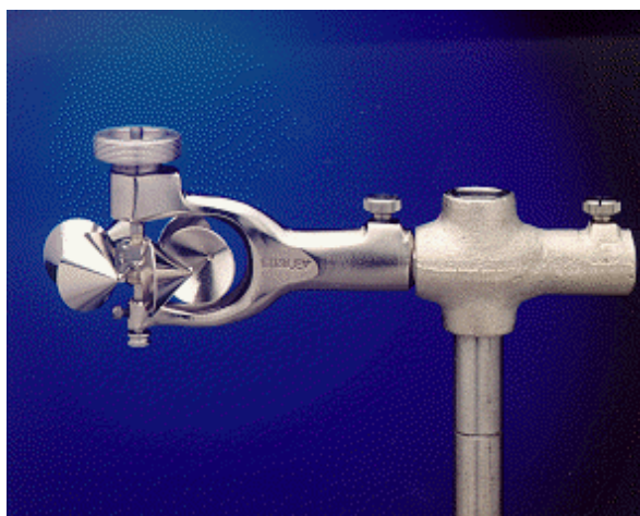
Figure 2. Gurley Pygmy flow meter (image/specifications table source: Gurley Precision Instruments http://www.gpi-hydro.com/ )
