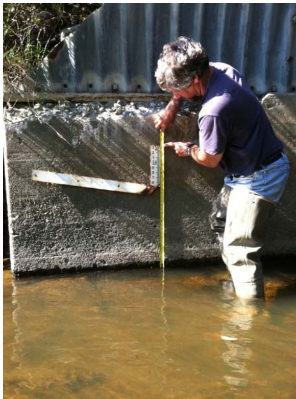
Figure 4. Measuring water level at established staff gauge
