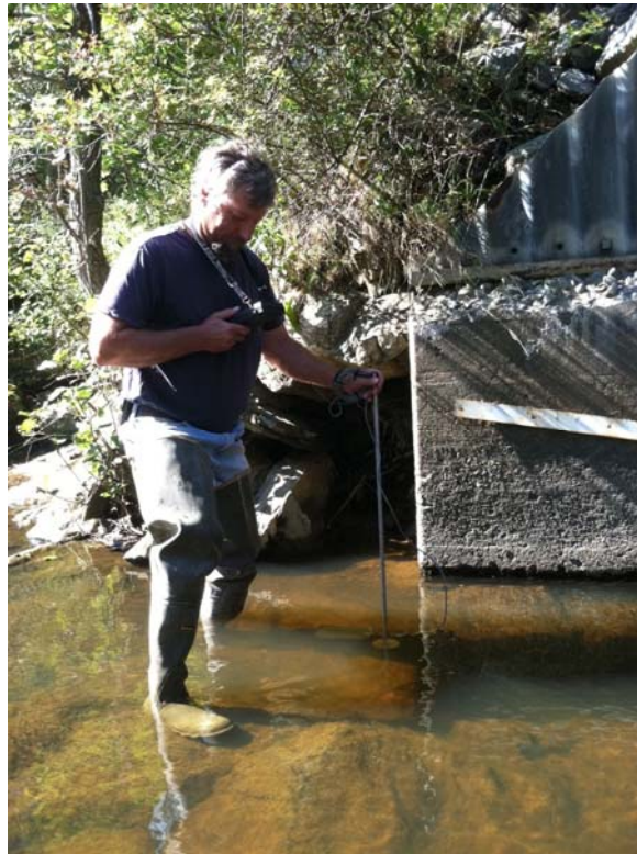
Figure 4. Measuring water level at established staff gauge
