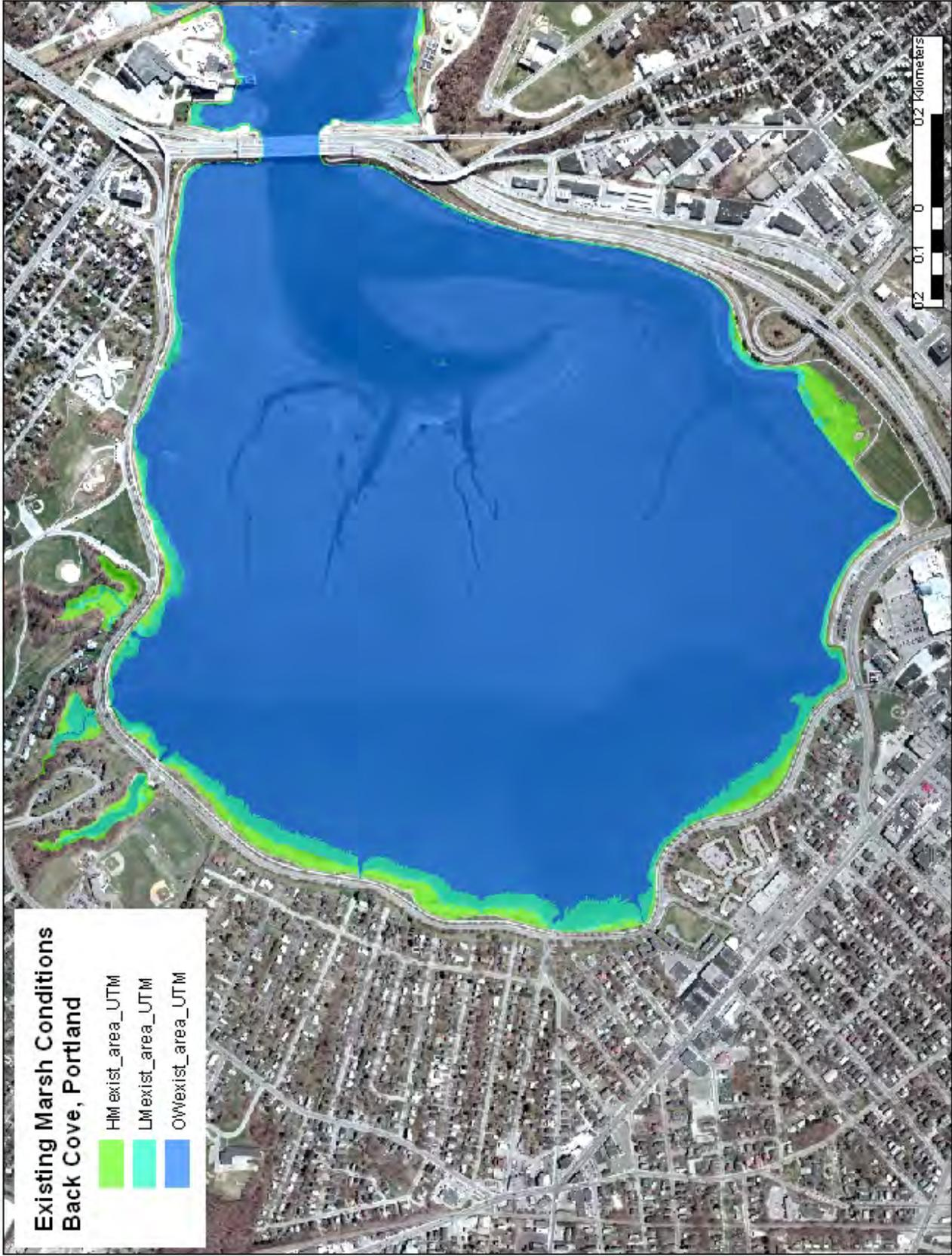
Figure 23. Simulation of existing marsh conditions at Back Cove using NOS tide data (NOS, 2009a). Note prevalence of fringing low marsh. An area of low lying uplands at the soccer field (lower right) is actually not existing marsh.
