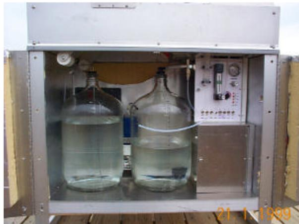
**Figure 2.** The interior of the dry collector
