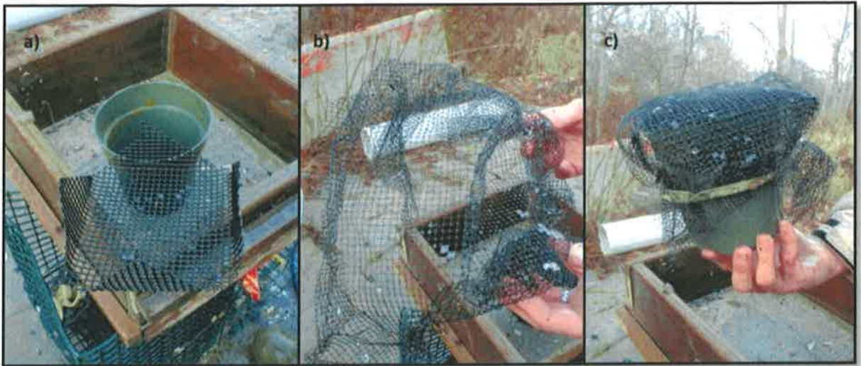
Figure 5. a) Experimental unit with piece of VEXAR; b) piece of 4.2 mm flexible netting that will hold the VEXAR in place on top of the unit; and, c) the experimental unit with the VEXAR and flexible netting held in place using a large rubber band. Treatment = FLEX & VEX.
