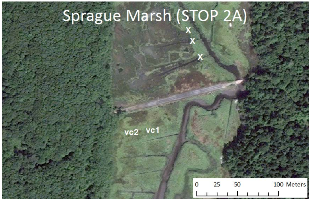
Figure 11. Points of interest for STOP 2A, including the causeway (road across the marsh) and “troll bridge” (eastern side of the causeway), location of ditch plugs (X), and location of cores taken (vc1, vc2) for stratigraphic cross section presented below and in Figure 12. (Satellite image taken 8/15/13.)
