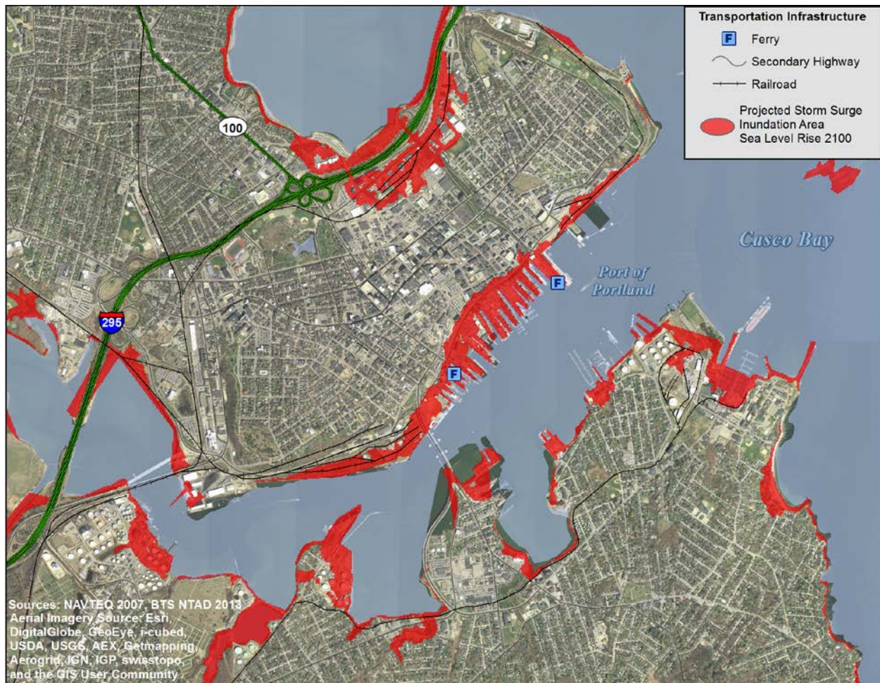
Figure 17 Storm Surge Inundation Impacts on Greater Portland Area Transportation Infrastructure
