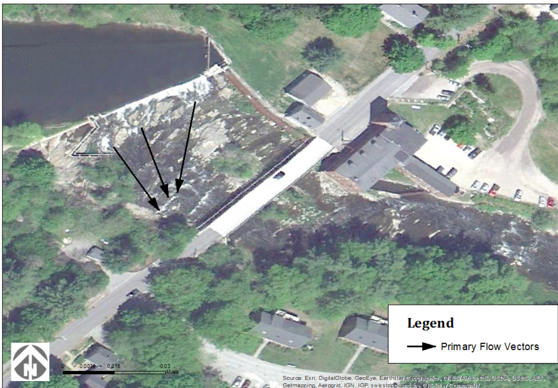
Figure 8: Site map of the Bridge Street site indicating primary flow vectors. Date of imagery is May 16, 2010. Flow direction is left to right.
