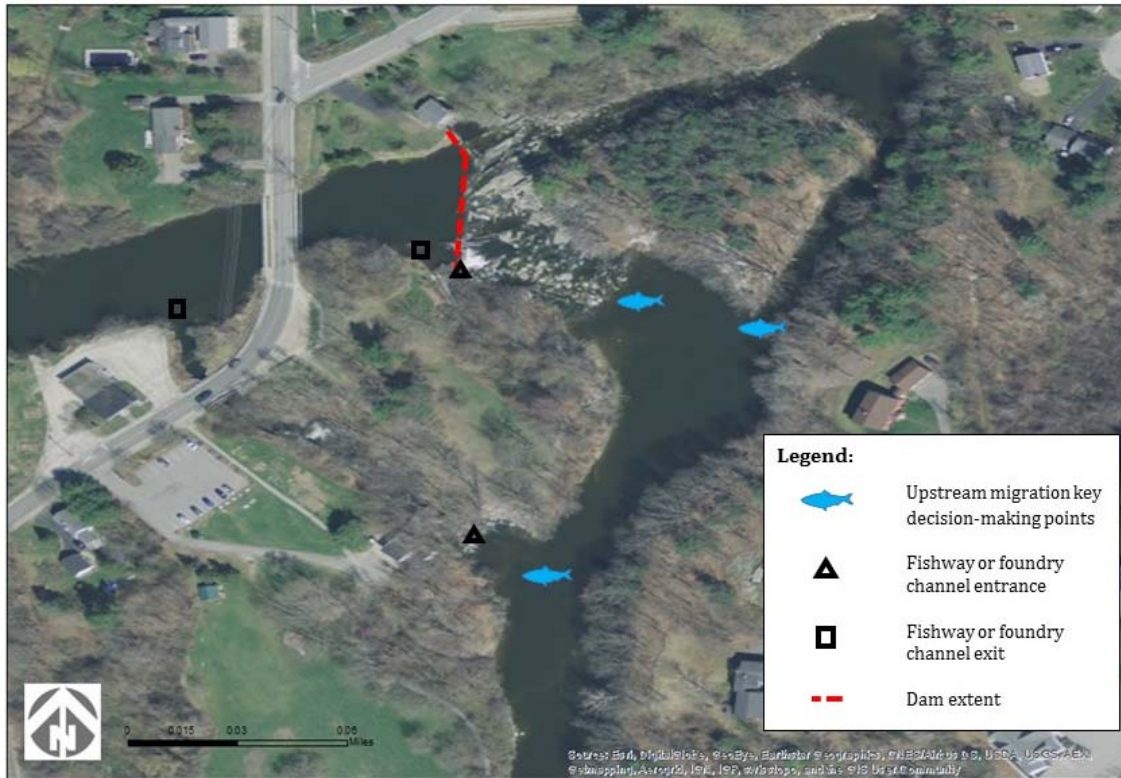
Figure 9: Site map of the East Elm Street site indicating key decision points for upstream migrating fish. Date of imagery is March 31, 2012. Flow direction is left to right at top of figure.
