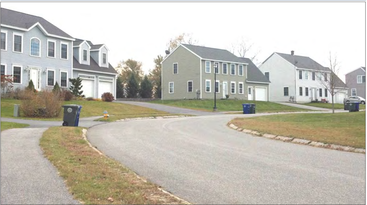
Impervious cover or hard surfaces include rooftops, driveways, sidewalks, and roads.
