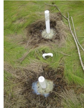
Photo 1. Typical cluster of Station wells.
