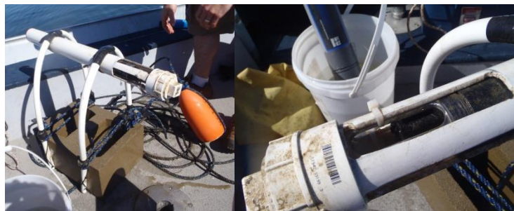
Figure 2. Marine example showing sonde in protective shroud attached to a frame and concrete anchor for bottom deployments (left), with focus (right) on sensor end.
