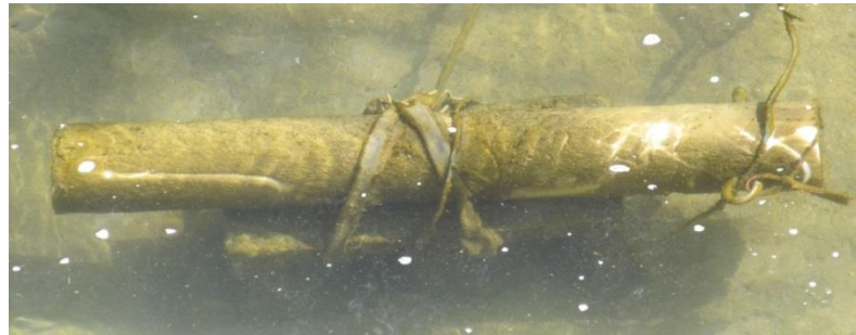
Figure 1. Algae and other fouling materials adhering to shroud and monitor. To protect monitors and reduce the need for abrasive cleaning, a shroud can be used to cover all or parts of the monitor.
