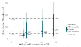
Impervious surfaces contribute to high chlorides. Even within the Long Creek Watershed, monitoring locations with more impervious surfaces upstream (draining subwatersheds with relatively more roads and parking) tended to have higher chloride concentrations over the period of record (2010-2018).
