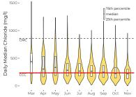
Daily median chloride concentration in Long Creek from 2010 through 2018 exceeded chronic exposure limits (CCC) over half the time. Conditions are generally at their worst in the spring, or under low-flow conditions. (Width indicates number of observations.)
