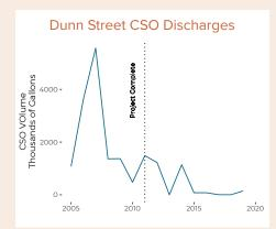
Discharges from the Dunn Street CSO dropped 85 percent after a larger pipe was installed and the weir modified
