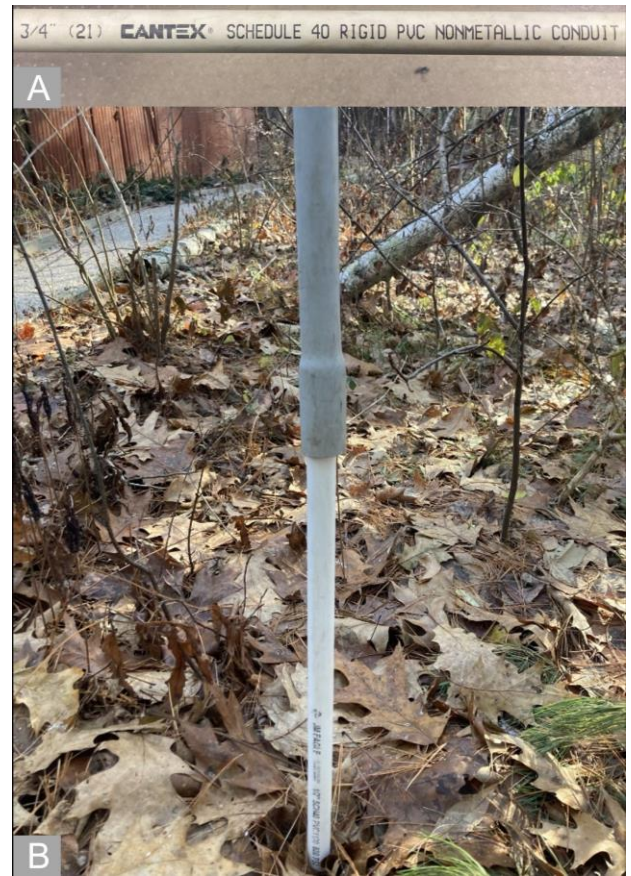
Figure 2. a) PVC Conduit pipe manufacturer details. b) The 3/4 inch conduit pipe fits onto the 1/2 inch pvc pipe.
